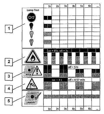
Fig. 14 Meaning of the signal patterns
